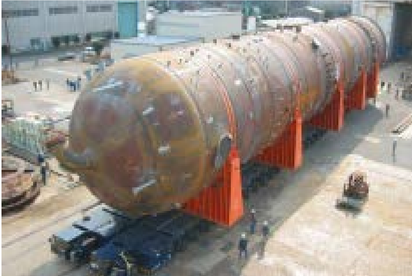
15,000 BBL/D Sasol F-T Reactor
